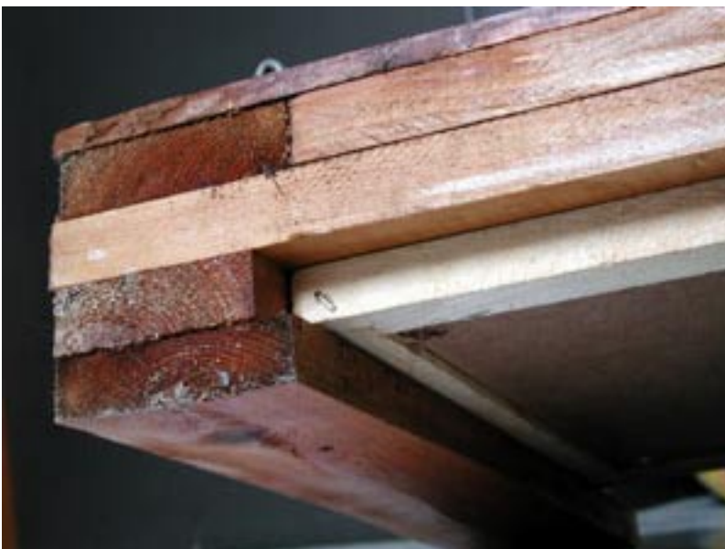
Figure 2: The sampling drawer slides into grooves on the supports of the bottom board
